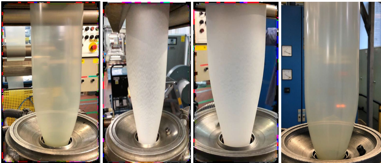
Fig. 29a–d: Visual appearance of the monofilm bubble (melt temperature):
