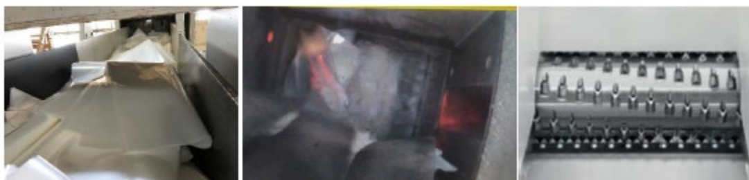
Fig. 25: S GRAN 95 impressions (left: material feed; middle: shredding unit; right: screw)
